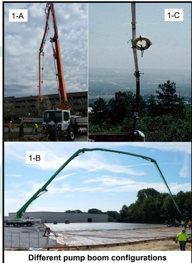
Different pump boom configurations
